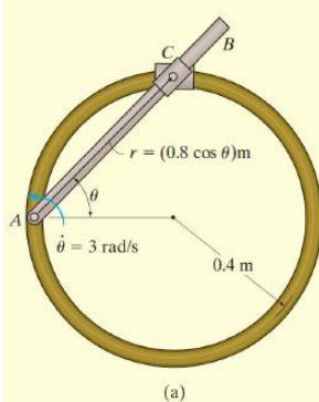
The smooth 0.5-kg double-collar in Fig. 13-19a can freely slide on arm  $AB$  and the circular guide rod. If the arm rotates with a constant angular velocity of  $\dot{\theta} = 3 \text{ rad/s}$ , determine the force the arm exerts on the collar at the instant  $\theta = 45^\circ$ . Motion is in the horizontal plane.
