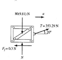
The crate has a mass of 80 kg and is being towed by a chain which is always directed at 20° from the horizontal as shown. Determine the crate's acceleration in t = 2 s if the coefficient of static friction is  $\mu_s = 0.4$  and the coefficient of kinetic friction is  $\mu_k = 0.3$  and the towing force is  $T = (90t^2)$  N, where t is in seconds.
